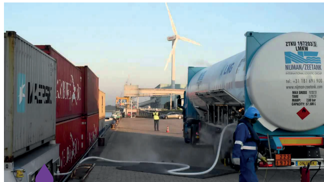
Avitaillement GNL «truck to ship», copyright Danser Group.
